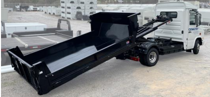
Switch-N-Go® system on electric chassis ⚡
