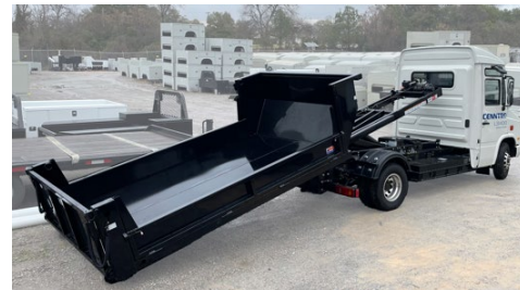
Switch-N-Go® system on electric chassis
