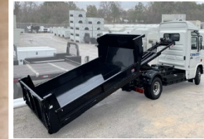
Switch-N-Go® system on electric chassis
